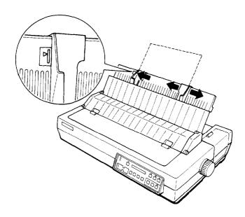
4. Slide a **sheet** of paper down between the edge guides until it meets resistance. At this time, the **PAPER OUT** light goes off.
